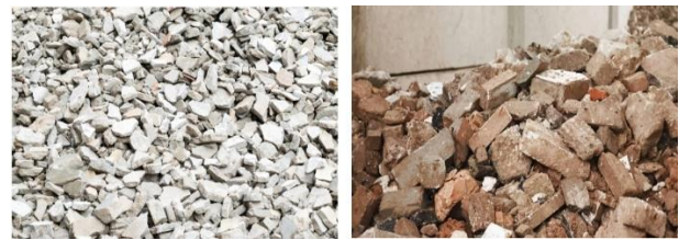
Figure 2. Sorted Demolition Waste on Site
