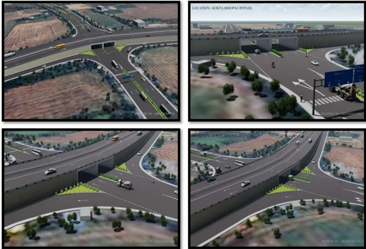
Figure 9. Modelling and Simulation of the proposed options have been done with the help of SketchUp software for better understanding and visualization.
