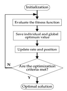
Figure.2 Particle Swarm Optimization Flowchart
