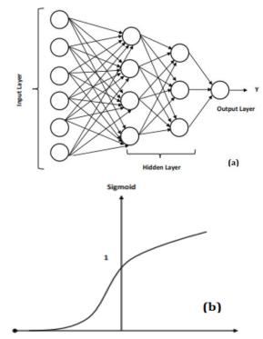
Figure 7. (a) Proposed neural network architecture. (b) Probabilistic curve of the sigmoid function.
