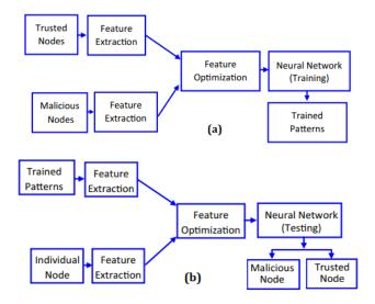
Figure 4 a Training Module of Intrusion Detection System. b Testing Module of Intrusion Detection System
