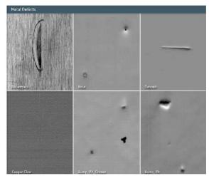
Figure 1 Surface Inspection, Precise Defect Classification images.
