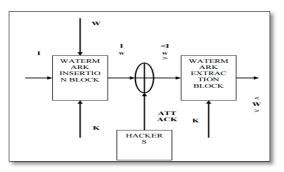
Figure 1 Generalized Model for a Watermarking System
