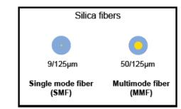
Figure 1. Two kinds of silica optical fibers based on their core/cladding diameters [1].
