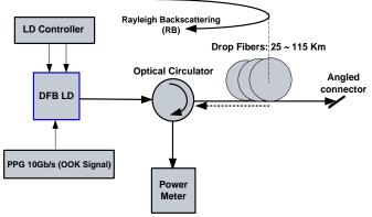
Figure 3. Experimental setup to measure the Rayleigh Backscattering (RB) noise in single fiber transmission.
