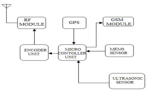
Figure.2.Block of robot section
