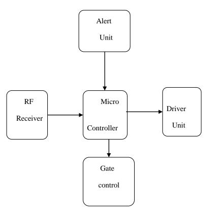
Figure.3. Block of gate control section
