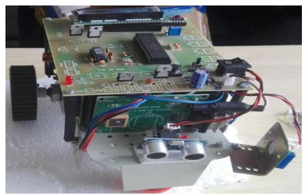
Figure.5.Snapshot of our designed robot control section
