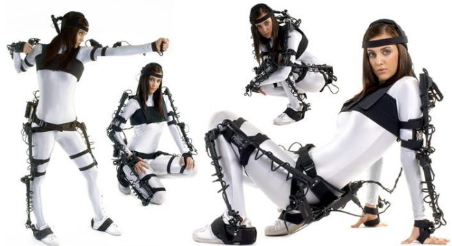
Figure 1 [8]. Mechanical motion capture equipment.
