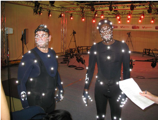
Figure 2 [6]. Optical motion capture equipment.
