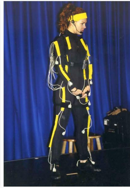
Figure 3 [6]. Equipment for electromagnetic motion capture.
