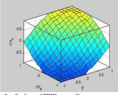
Fig.3: - Surface of FPID controller
