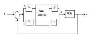
Fig.1. The PID type fuzzy control system
