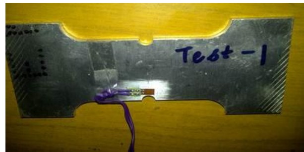
Figure 3 Positioning of strain gauge
