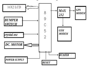
Figure.4 Block Diagram for walker type system
