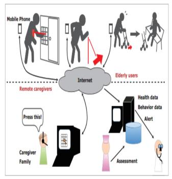
Figure. 2. Safety navigation system overview. Elderly users can get support with laser projection-based indication from remote caregivers.
