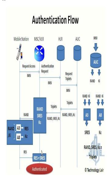
MNO checks the validity of SIM. It decrypts Ekc(R||Rs) using Kc.MNO compares R with R in response. If both are
