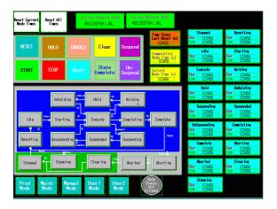
Figure 2 - Example display of machine mode and state models
