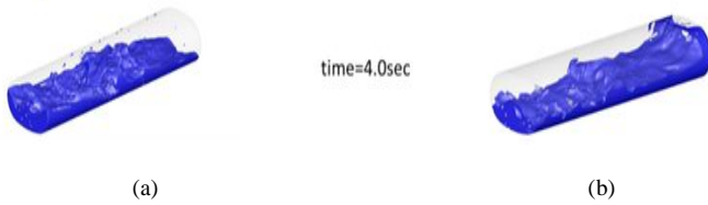
Fig 15 Comparison between CFD results of (a) without baffle (b) with baffle at t=4 sec after applying break
