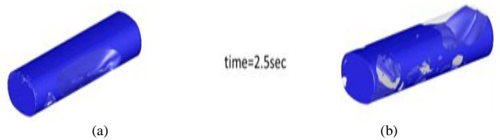
Fig 12 Comparison between CFD results of (a) without baffle (b) with baffle at t=2.5 \text{ sec} after applying break
