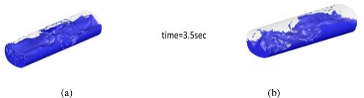
Fig 14 Comparison between CFD results of (a) without baffle (b) with baffle at t=3.5 \text{ sec} after applying break
