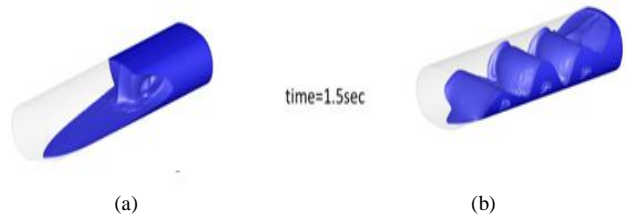
Fig 10 Comparison between CFD results of (a) without baffle (b) with baffle at t=1.5 \text{ sec} before applying break
