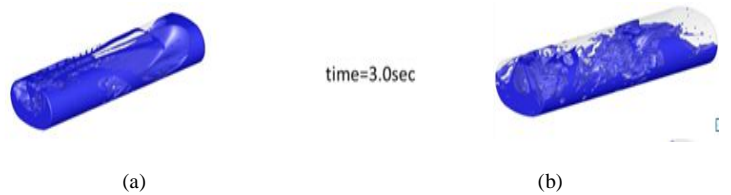
Fig 13 Comparison between CFD results of (a) without baffle (b) with baffle at t=3.0 \text{ sec} after applying break
