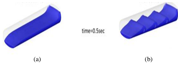
Fig 8 Comparison between CFD results of (a) without baffle (b) with baffle at t=0.5 \text{ sec} before applying break
