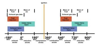
Figure 2 The control event of a SI engine.
