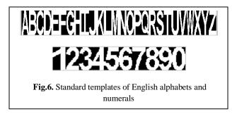
Similar process is used to segment the characters from the test image. Each character is matched with the standard template using correlation technique to measure the similarity between them using equation.1. Correlation coefficient value ranges from 0 to 1. The value 0 indicates minimum match and value 1 indicates maximum match.
