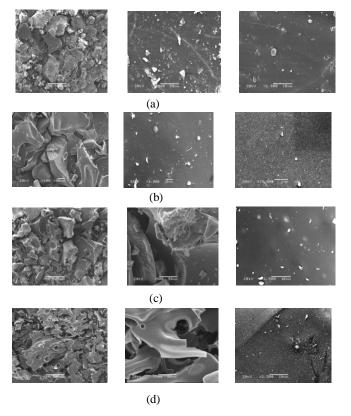
Figure.3 SEM for physically treated chicken feather surface atdifferent carbonization temperature :(a) 200 °C(b) 300°C(c) 400°C(d) 500°C
