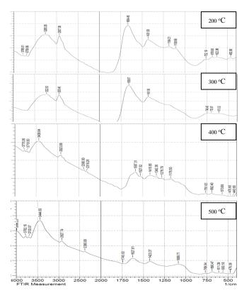
Figure .5 FTIR comparison curve of physically treated chicken feather at different Carbonization temperature
