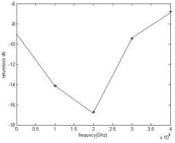
Fig 2 Return loss vs. Impedance match as a function of frequency plot (MATLAB)
