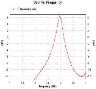
Fig 10 Gain vs Frequency plot From fig 10 we find that maximum gain occur at 2.58Ghz frequency
