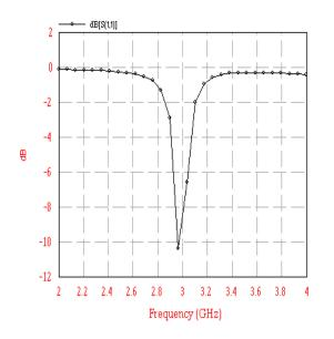
Fig 8 Frequency vs. return loss patch of L-slit antenna
