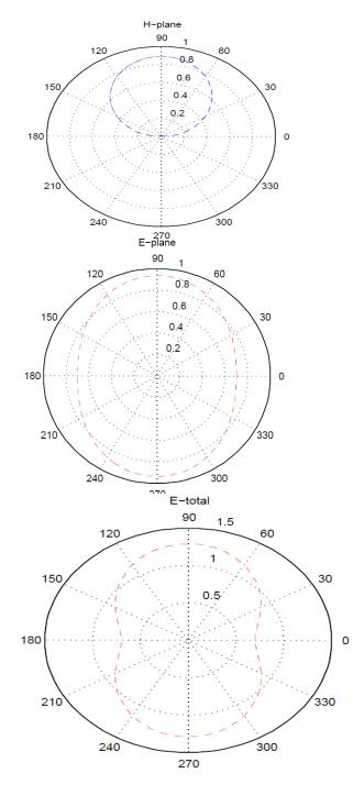
Figure 4: Radiation patterns at (a) E-plane and (b) H-plane (c) E-total
