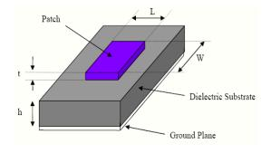
Fig-1 Structure of a Micro strip Patch Antenna
