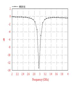
Fig 7 Frequency vs. return loss patch
