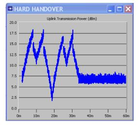
Fig.6 Uplink transmission power for hard handover
