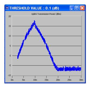
Fig. 11 Uplink transmission power for threshold value 0.1 dB
