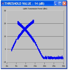
Fig. 15 Uplink transmission power for threshold value 14 dB
