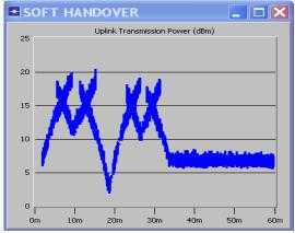
Fig.7 Uplink transmission power for Soft Handover
