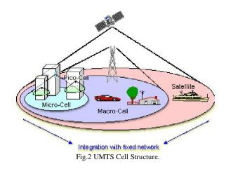
Higher levels cover larger geographical areas. Lower levels cover only little areas but they can handle a higher density of devices that want to access the network in this little areas. They also provide faster wireless links to the network than larger levels. The whole system is connected and integrated with PTSN (Public Telephone Switched Network) and PDN (Public Data Network) like internet etc [3]. The following levels are planned:
