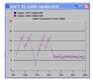
Fig.8 Comparison of uplink transmission power between hard handover and soft handover
