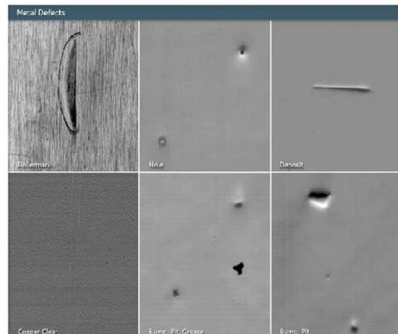
Figure 1 Surface Inspection, Precise Defect Classification images.
