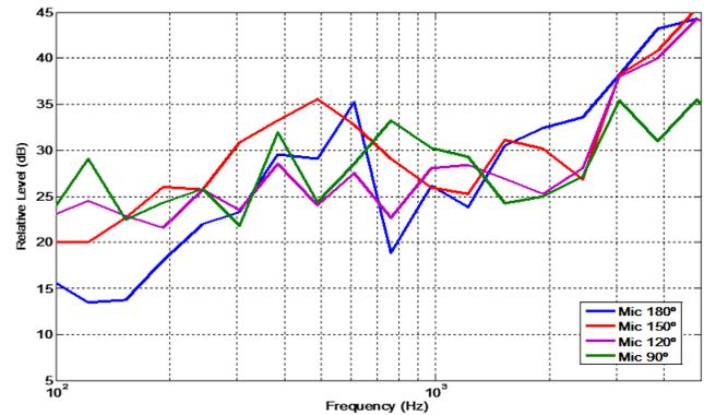
Figure 11. Frequency dependence of TL through the engine hood for different angles
