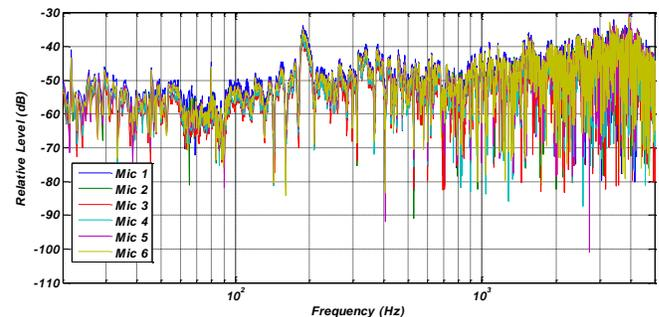
Figure 3. Transfer function of the data acquisition system
