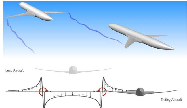
**Figure 5. Wake downwash/upwash from a leading aircraft [14]**
