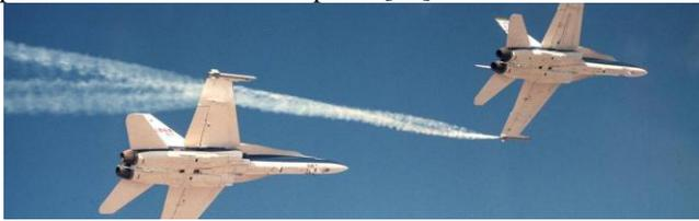
**Figure 6. Autonomous Formation Flight (AFF)**
