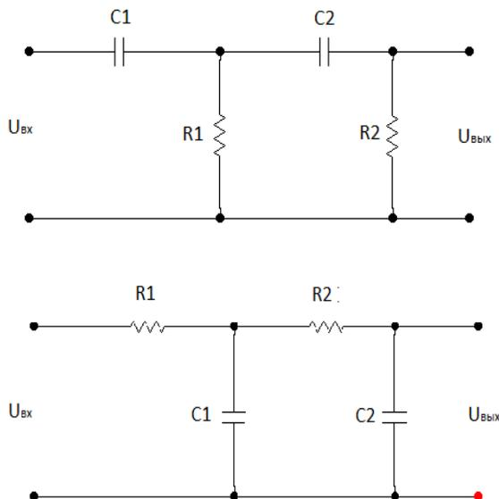
Fig.5. Phase-rotating chains
