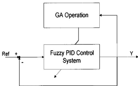
Fig.5: - GA operation on FPID controller
