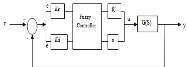
Fig.1. The PID type fuzzy control system
