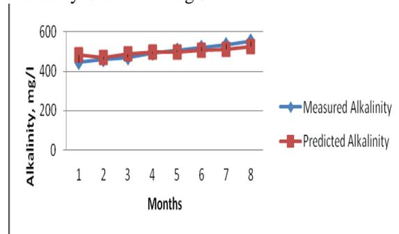
Fig.3 comparison between measured alkalinity and predicted alkalinity, M3.
