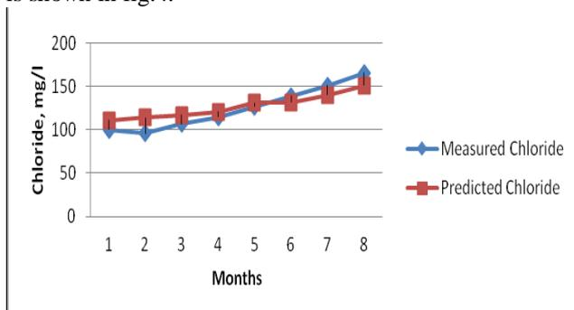
**Fig.4 comparison between measured chloride and predicted chloride, M4.**
