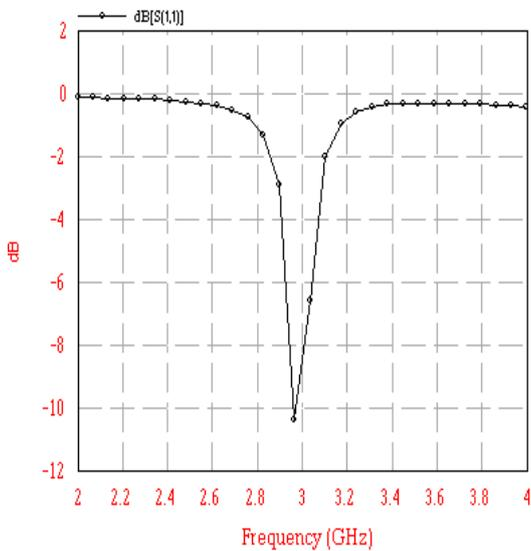
Fig 8 Frequency vs. return loss patch of L-slit antenna
