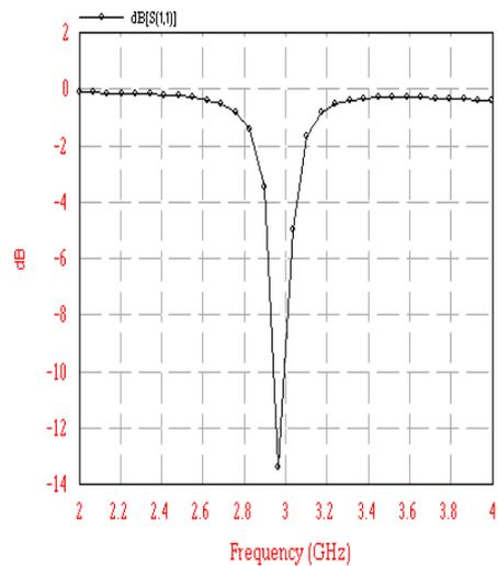
Fig 7 Frequency vs. return loss patch
