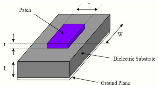
Fig-1 Structure of a Micro strip Patch Antenna
