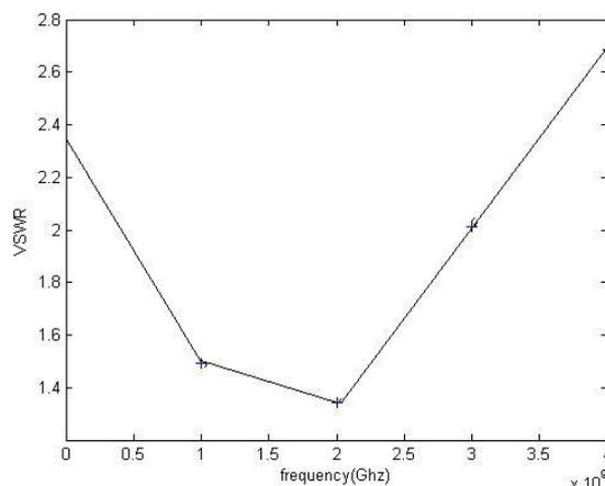
Figure 3 shows the impedance match as a function of frequency vs. VSWR
