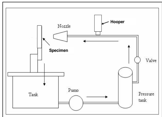
Fig 1: Schematic High Velocity test rig for sand erosion
