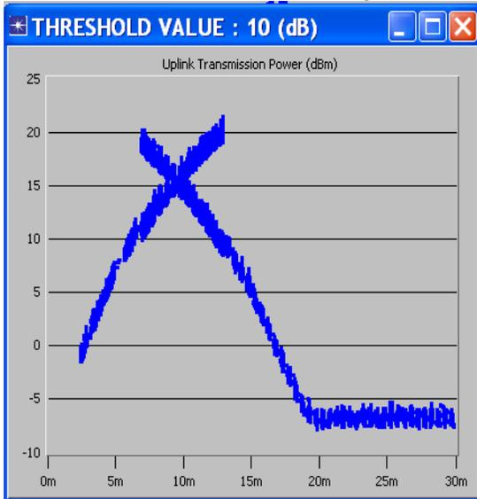
Fig.14 Uplink transmission power for threshold value 10 dB.
