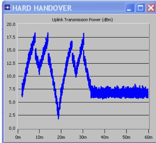
Fig.6 Uplink transmission power for hard handover
