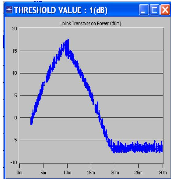
Fig. 12 Uplink transmission power for threshold value 1 db.
