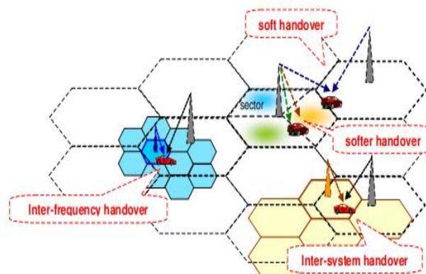
Fig.4 UMTS Cell Architecture
