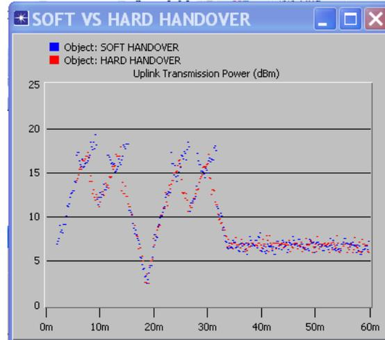
Fig.8 Comparison of uplink transmission power between hard handover and soft handover
