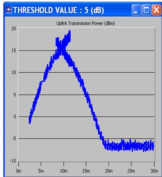
Fig. 13 Uplink transmission power for threshold value 5 dB
